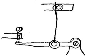
Steel rod heated expands and regulates its own circuit
