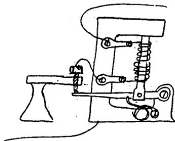
Platina spiral heated to incandescence expands a zinc rod so as to open and control circuit. This works well but gets hot making one larger<sup>1</sup>
