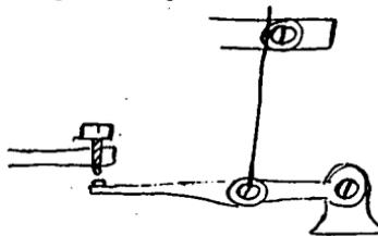
Platina rod heated to incandescence expands and opens its own circuit. This regulates very rapidly
