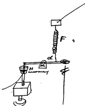
In figure 23 is shown a spiral F which when it expands throws up the lever, d & breaks contact in the mercury cup .H.
