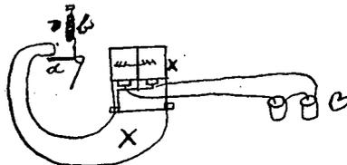
Fig 34 shows an electric or other engine with a fan to produce a draft of air to cool the spirals the draft being regulated by the lever d closing the draft tube .X.
