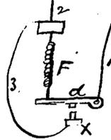
Fig 25 shows it arranged to short circuit the spiral when the temperature is too high the point X may be provided with a spring so that the spiral will not be affected when pressing the lever downward as it would if a rigid point were used.
