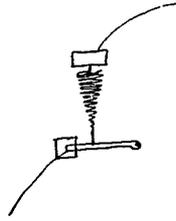
Fig 31 shews a spiral which when not heated has a portion of its spiral touching each other and thus out of action upon the passage of the current more and more spirals and consequently resistance is thrown in circuit by the expansion of the same
