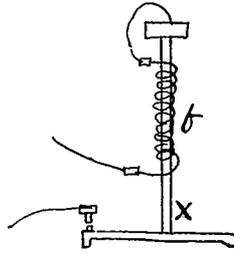
Fig 35 shews the passage of the current through both the spirals F and expanding lever X thus working it by both direct and radiant heat. the short circuiting device may be used in this arrangement.
