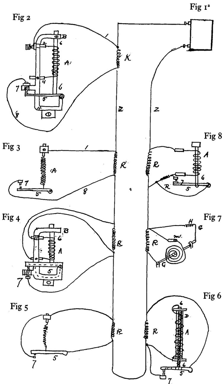
Fig 1 is a magneto electric machine supplying currents to a circuit Z-Z.<sup>3</sup>
