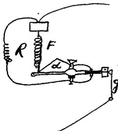
Fig 29 shews a spiral making<sup>b</sup> a lever having two contact<sup>11</sup> 1 and 2 on its extremity insulated from each other. a spring  $g$  is either in contact with one or the other as the spiral is expanded or contracted thus opening or closing the circuit through the spiral or through a resistance  $R$  equal to it but of large wire to prevent heating.
