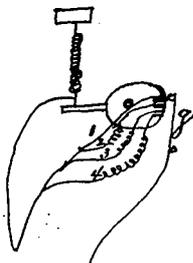
Fig 30 shews a similar arrangement except that as the spirals tends to elongate more and more it is checked by throwing in constantly increasing resistances 1. 2. 3. & 4
