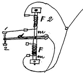
Fig 27 shews a double spiral<sup>10</sup>  $F_1$  &  $F_2$  with lever  $d$  connected to the expanding rods  $m$  and  $m'$  arranged with contact
