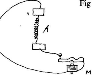
In figure 6. a glass tube d passes through the centre of the spiral—A. through this tube passes the expanding rod 6. The operation is the same as in figure 4 but it is a more convenient device.
