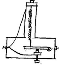
Fig 42 shews a spiral with self regulator inclosed in a glass tube.
