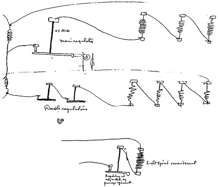
16. The following day Edison sketched some ideas about generators, including a tuning-fork generator (Vol. 16:16, Lab. [TAEM 4:406]). The tuning-fork design, labeled "Magneto machine with fork," modified his tuning-fork motor to create a direct-current generator (see Docs. 782, 800, and 802). Steam from the boiler (right) drives two double-acting pistons, located on opposite sides of the tuning fork near the top of each prong, vibrating the fork. As the electromagnets attached
