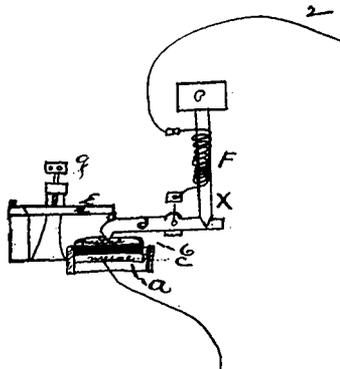
In figure 21. C is a button of finely divided conducting matter that varies its resistance by pressure. This button is placed between two metallic armatures<sup>7</sup> A & B. D is a lever which is pressed down upon the armature B by the spring E aided by the screw .g. X is a rod of material quite expansible by heat
