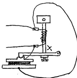
In figure 22 The arrangement is somewhat different. the expansion of the rod X by the heat of the spiral increases the pressure and decreases the resistance of the button hence cuts off more current from the spiral, thus reducing its temperature.
