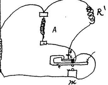
In figure 16 a thermoelectric pile X is placed in close proximity to the heated spiral the current from it actuates a magnet M whose lever N and point O opens and closes the shunt containing the spiral A, when the temperature of the spiral becomes too high the current generated by the thermopile causes the magnet M to attract its lever and open the deriva-
