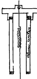
Fig 40 shows double tubes the spaces between being filled with a solution of Alum in water to further decrease conduction and radiation of heat.
