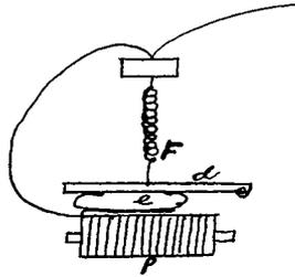
Fig 32 shows a method of gradually increasing the power of the shunt on short circuit. P is a cylinder wound with wire offering considerable resistance. E is a spring which when just touching P comes in contact with but few spirals and as the temperature of the spiral increases the spring e flattens and comes in contact with more convolutions hence shunting more and more current from F
