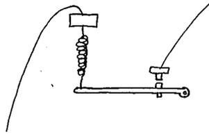
Fig 24 shews the expansion of the spiral opening its own circuit and the contact point being placed near the fulcrum to gain power.
