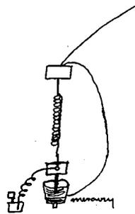
Fig 26 shews a spiral with slight weight short circuiting itself in a cup of mercury or on a spring.
