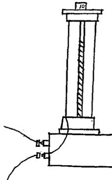
Fig 43 shows a spiral wound around a pencil of lime or similar substance to accumulate heat and thus render the spiral incandescent with much less strength of current—
