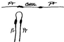
we took a piece of 6 cord thread No 24s which is about 13 thousandths in thickness and after fastening to Pt wires we carbonized it in a closed chamber. we put in a bulb and in vacuo it gave a light equal to about 1/2 candle 18 cells carbon. it had resistance of 113 ohms at starting & afterward went up to 140— probably due to vibration<sup>a</sup>
