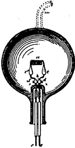
*The drawings for Edison's 1 November patent application (U.S. Patent 223,898) show the ends of the filaments c c' thickened with lampblack and tar. At this point Edison still preferred the spiral shape as a way of increasing resistance and reducing radiating surface.*
