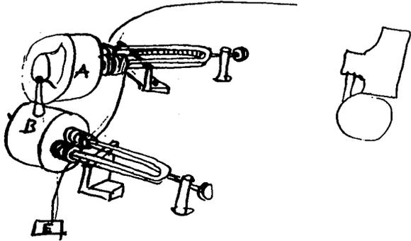
Conveying air to the second Telephone through tube in manner shewn sets diaphragm of B in powerful vibration at each wind sound or hiss the vowel & musical sounds be obtained from .A.
