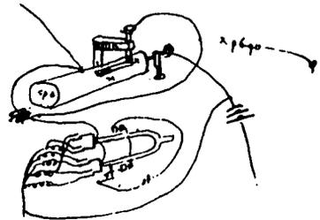
A hiss produces a wind pressure in tube & this raises n with more or less pressure against the plumbago point X this throws in a hiss sound produced by a tuning fork arranged to give a number of Contacts 1 after the other. <sup>b</sup>
