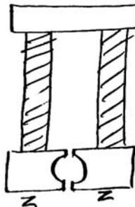
Cores 24 inch long Cores 4 in thick Put the machine on the wooden base used by big induction magnets before & fasten down by Z<sup>4</sup> see book 46. 105 page<sup>5</sup> <Completed April 12th 79 J Kruesi><sup>6a</sup>
