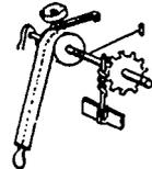
Fig. 63 shows a pull strip upon which the indentations are, pulling the strip downward, winds up a rubber elastic; when the strip is let go of the worm and fan regulates the power of the elastic.
