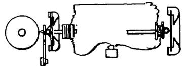
When it is desired to record speech from a distance, I arrange it as in Fig. 10; an electro-magnet in the line serves to give motion to the indenting spring directly or from a diaphragm.
