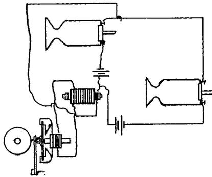
with the induction coils and batteries with these collectors and convey wires from each coil to a common magnet working the indenting point.
