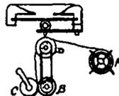
Fig. 43 shows a long strip or roll like that of a Morse register. A is a roll of the material, D the drum, B the reel upon which the material is wound, C, a roller which keeps the material smoothly on B.
