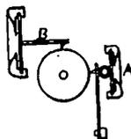
Fig. 40 shows both a recorder A, and a reproducer B. A acts direct, while the lever of B cannot of itself indent the foil, yet falls into the indentations made by A.
