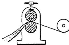
Fig. 57 shows a method of preparing bands of material already indented with the proper indentations for reproducing any kind of sounds, one roller having an original made by coating-tin foil with copper and then steel, or making a plaster of
