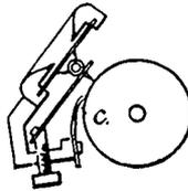
Fig. 83 shows an extra point c, for slightly grooving the foil before the indenting point; this takes part of the work off the indenting point.
