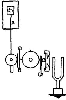
Fig. 79 a method of recording the sound, and<sup>d</sup> tuning-forks and obtaining their vibrating time, X being a pendulum to give the time.
