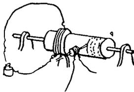
then when an indentation passes the point the attraction will be less than when no indentation passes; this will give good articulation, free from the scraping noise of the point on the foil, for in this case it does not touch the foil, but is worked by magnetic attraction.
