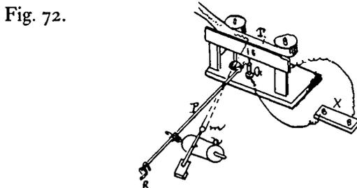
Fig. 72 shows a method of amplifying the records and photographing the same; n is the cylinder containing the indentations; m a small mirror; G a stand holding an electric or other light which passes through a slot 3 to the mirrors m, and is reflected back upon the paper T, which, with the cylinder N, is rotated by a shaft P, handles R, and worm at each end.
