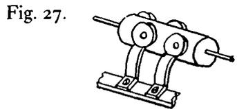
Fig. 27 shows another arrangement whereby several persons may speak simultaneously, but their record will be in separate spirals, the cylinders being provided with double thread or spirals.
