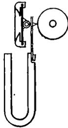
in which the spring-arm of the reproducing point connected to the diaphragm is highly magnetized, or the iron-foil may be magnetized, as in Fig. 14;
