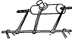
Fig. 45 shows an indenting and reproducing apparatus carried back and forward automatically by a double thread, one right hand on the front and left hand on the back of the machine.
