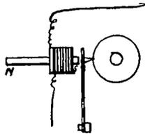
When the carbon telephone is used, the spring is connected by a piece of rubber tubing to the two platina discs between which is the carbon all placed in a circuit containing a battery and receiver, as in Fig. 9. Of course, the line may be of any required length with complete apparatus at each end, the phonograph merely replacing the person talking.
