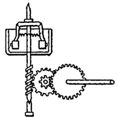
X, Figs. 16 and 19, is a plate revolved horizontally by a train of gear as shown in Fig. 21; this plate has two volute spirals cut from the center outward; the inner spiral 11, Fig. 16, is used for the purpose of carrying the arm A outward; this arm has upon its extremity the diaphragm and guide or carrying arm n;<sup>3</sup> the other spiral 12 is used to lay the foil or material
