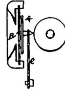
A small disc A, of mica or other stiff and light material is secured to the spring e, Figs. 6 and 7, which disc is immediately opposite the diaphragm B (Fig. 7), but not touching the air waves serving to give the requisite motion.
