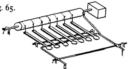
Fig. 64 is similar to 62. Fig. 65 is a cylinder and key board, around the cylinder opposite the keys are the necessary indentations to form a letter of the alphabet or a tone or note of the scale.
