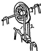
Fig. 41 shows a plate with spirals cut on each side with double reproducers, 1 and 2. This will be useful in toys, the sentence or sound being indented permanently on each side of the plate and the arms 1 and 2 being thrown in and out automatically.
