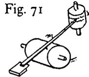
Fig. 71 shows a method of obtaining amplified records from the indented sheet. M is the lever, X a lamp-blacked cylinder; both are rotated slowly.
