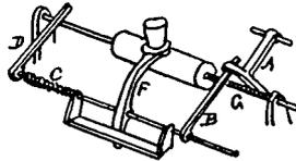
Fig. 46 shows an automatic machine suitable for advertising purposes: the arm F is carried forward by the screw G, in going forward it lifts up A, until A drops back, then the spiral spring, c, causes B to run over A, back to its starting point again.
