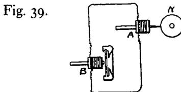
Fig. 39 shows a cylinder which has upon it iron-foil, indented by a separate mouthpiece. A is a permanent magnet close to the indentations; around the magnet is a coil of wire. B is a polarized receiving instrument. The rotation of N causes the indentations to throw inductive currents into B, and thus reproduce the speaking or other sounds; although the point of A does not touch N, the approach and recession of the iron causes the currents to be set up.
