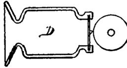
being used to collect the sound; this it does with great power; several of them may be connected together; another plan is to use several chambers in different parts of the room and connecting by tubes to the recording diaphragm; still another plan is to connect several of my carbon telephones, Fig. 12,
